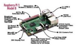
Fig.1: Raspberry Pi 3 Model B
